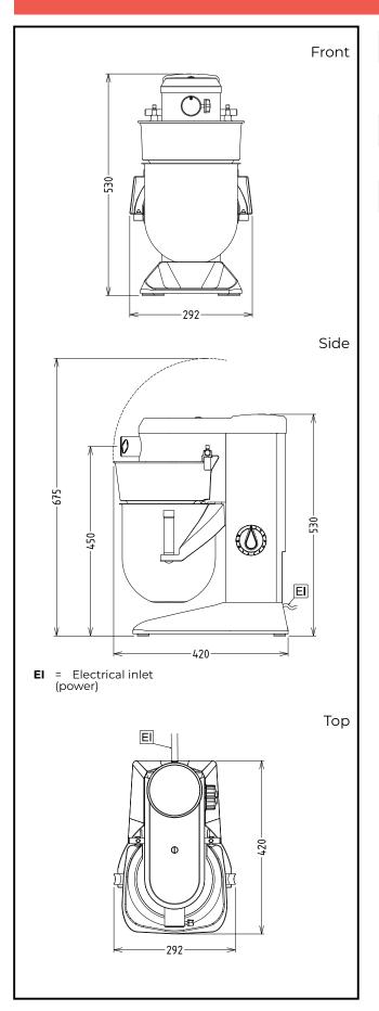
Electric Supply voltage: 200-240 V/1N ph/50/60 Hz Electrical power, max: 0.6 kW **Total Watts:** 0.6 kW Capacity: Performance (up to): 2.5 kg/Cycle Capacity: 8 litres Key Information: External dimensions, Width: 292 mm External dimensions, 416 mm Depth: External dimensions, Height: 527 mm **Shipping weight:** ISO 9001; ISO 14001 kg Net weight (kg): **Cold water paste:** 2.5 kg with Spiral hook
